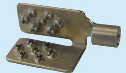
The crimp tool compresses the connector to the round feed cable and clamps the teeth of the crimp onto the copper tape. There are three different types of crimps, two for different gauge wires (10-12AWG and 14-16AWG) and one for extending lengths of copper tape (Termi-foil splice crimp).
