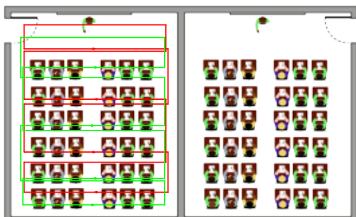
Larger room with metal in floor structure and a requirement to prevent overspill.
